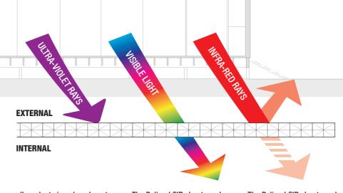
all products in polycarbonate by dott. gallina are UV protected and block out the harmful ultraviolet radiation
